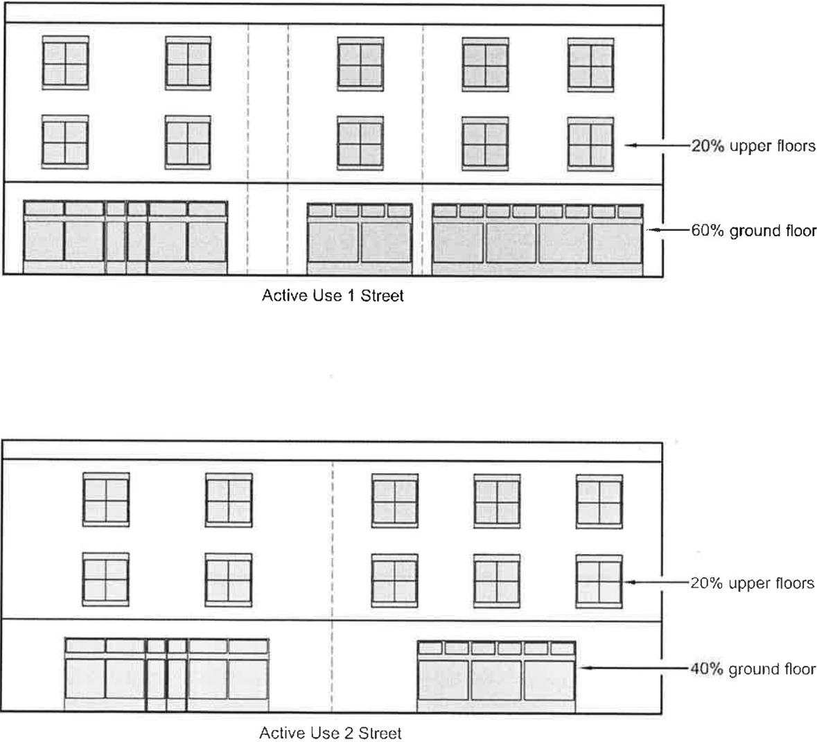
**Figure 11 - Example of Building Façade Transparency in the R-24 NB and R-25+ NB Districts (Elevation)**
