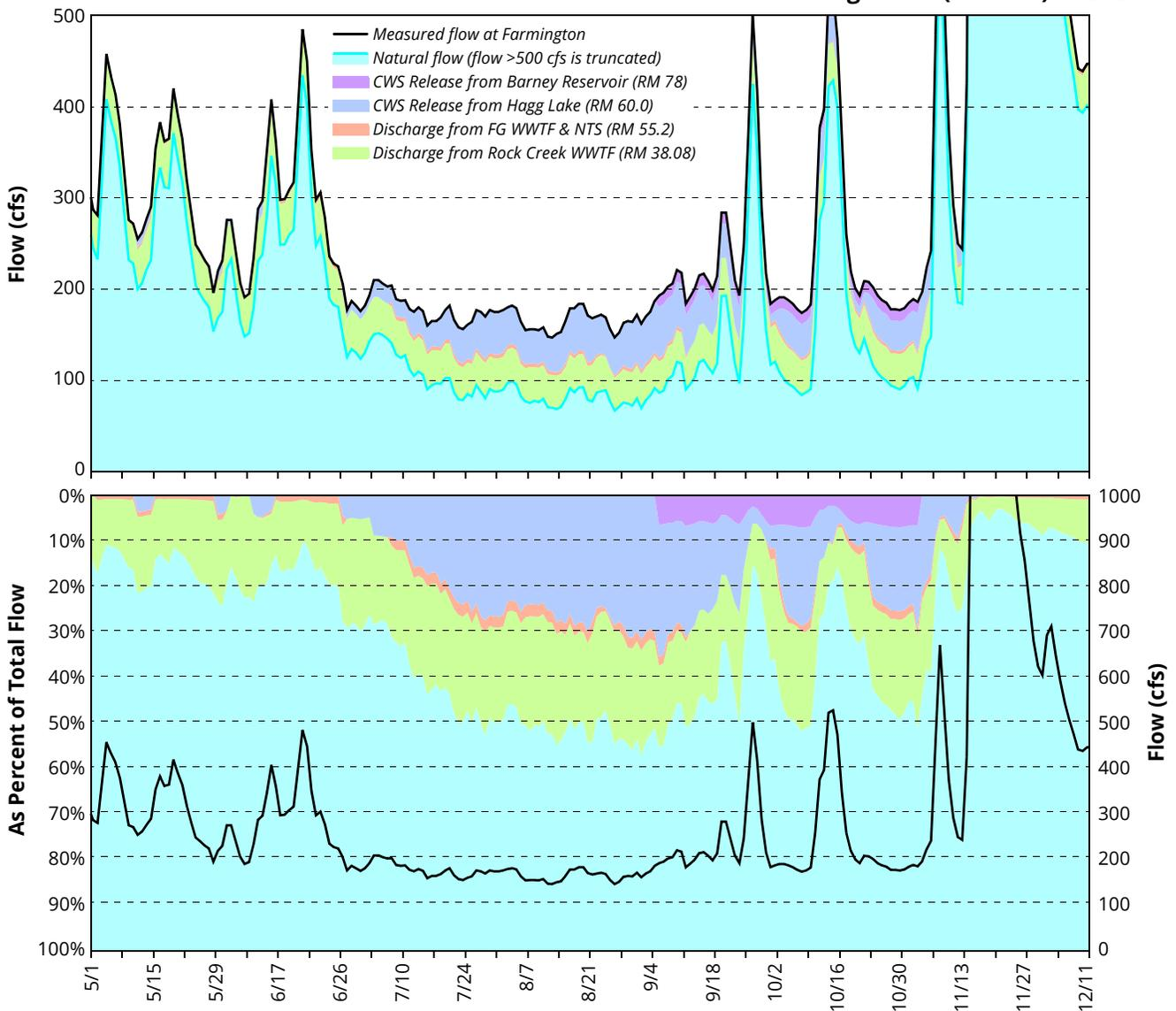
\*The following formula was used to calculate flows in this figure, assuming constant travel time and a uniform evaporative loss (0.25% per mile).
