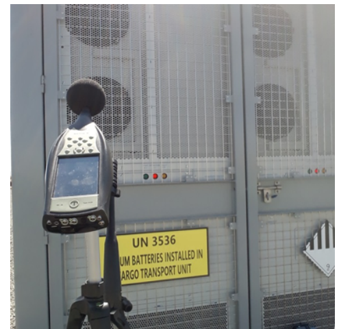
Our detailed noise measurements of a battery unit included obtaining directivity and spectral data.
