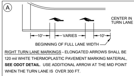
**RIGHT TURN LANE MARKINGS** - ELONGATED ARROWS SHALL BE 120 mil WHITE THERMOPLASTIC PAVEMENT MARKING MATERIAL, **SEE ODOT DETAIL**. USE ADDITIONAL ARROW AT THE MID POINT WHEN THE TURN LANE IS OVER 300 FT.
