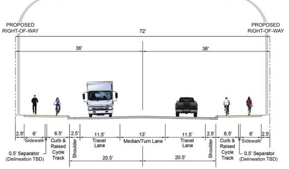
Note: Temporary construction easements and/or permanent easements may also be necessary beyond the proposed right-of-way limits shown.
